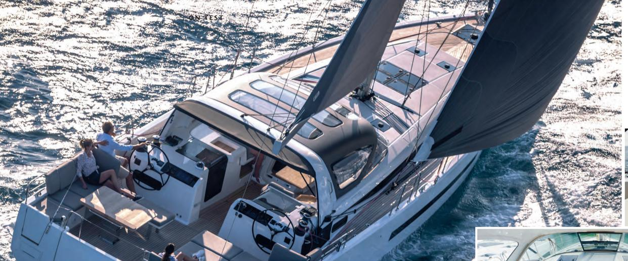
Left: a pair of electric winches at each helm station allow for push-button sail handling.
